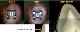
Example of before and after images and erosion [T-XT sample #5]
